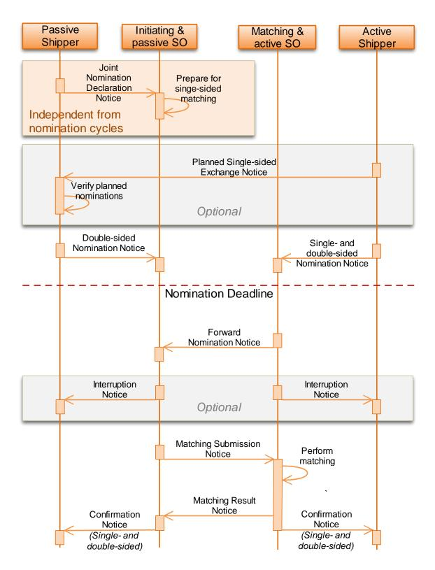
The following sequence diagrams summarise the nomination and matching process if the matching system operator is the passive system operator.
